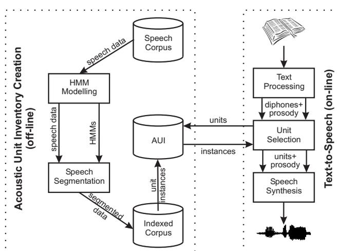
Fig. 1. Block diagram of ARTIC TTS system.
