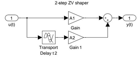
Fig. 5. Schematics of 2-step ZV filter in Simulink.
