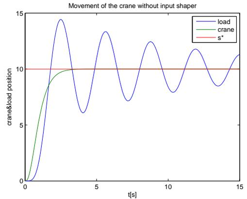
Fig. 6. Movement of the crane without ZV-filter.
