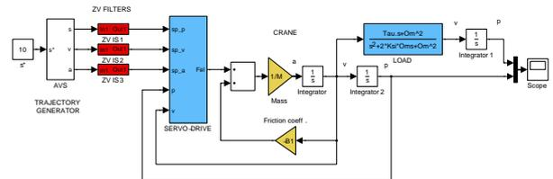
Fig. 10. Schematics of the crane with electrical drive and t-optimal trajectory generator (block AVS) in Simulink.
