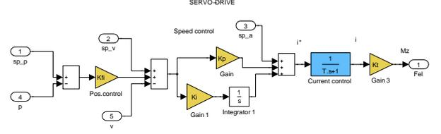
Fig. 4. Schematics of the electrical servo drive in Simulink.
