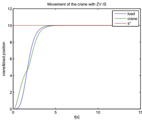
Fig. 8. Movement of the crane with ZV-filter.
