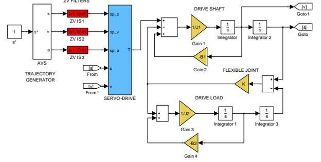
Fig. 14. Schematics of the flexible shaft with the electrical drive and ZV filter in Simulink.
