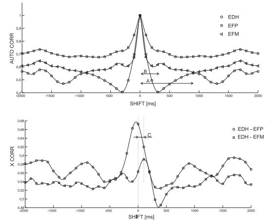
Fig. 5. The upper figure depicts auto-correlation separately for energy dominant hand:  $EDH$ , face pose:  $EFP$  and mouthing:  $EFM$ , the lower figure shows cross-correlation between energy of manual and non-manual component only.
